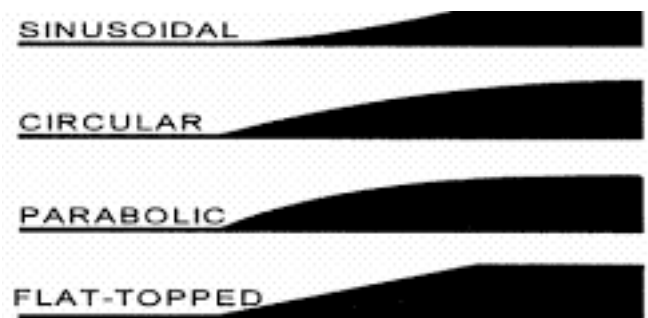
Figure B-20: Speed Hump/Cushion Profiles
