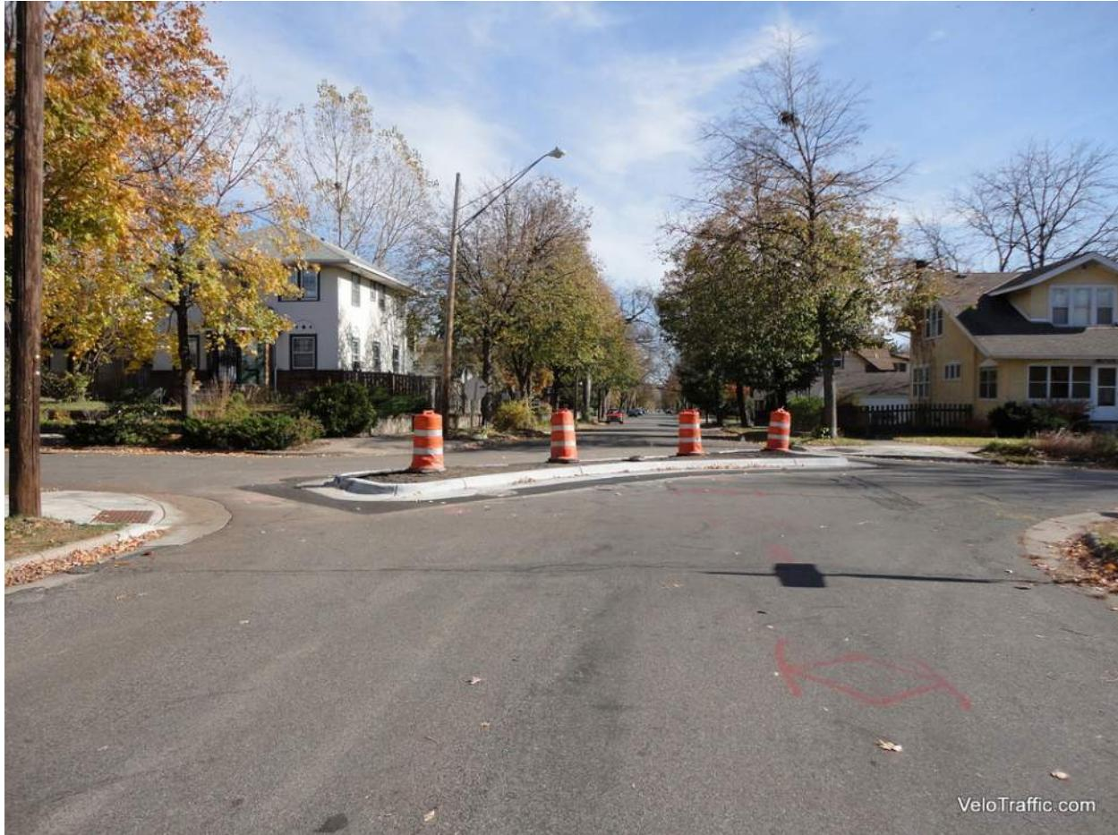
Diagonal diverters are barriers built diagonally across the middle of an intersection, preventing through and/or turning movements. Pedestrian and bicycle traffic are usually unrestricted.
