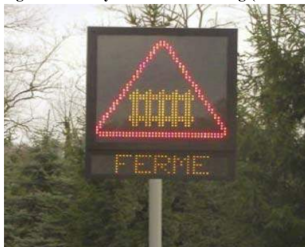
Figure 2-9 VMS in Protected Crossing (Ref. 2-6)
