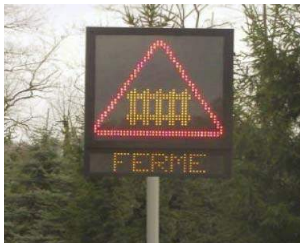
Figure 2-3 VMS in Protected Crossing (Ref. 24)
